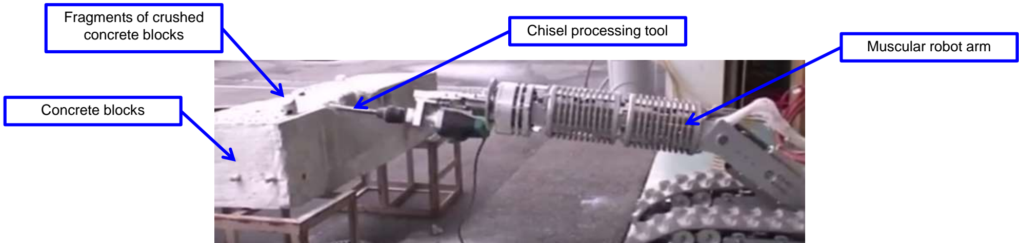
Concrete block crushing test by a chisel processing method
