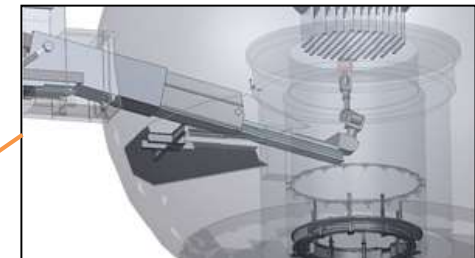
Verifying maneuverability by a combination of a robot arm and access rail
